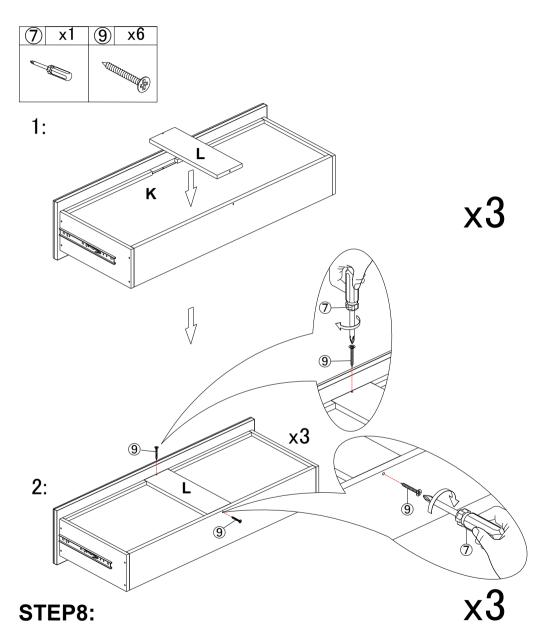
Insert panel(L) into preassembled unit at step 7, use screws (9) to attach them as picture show, tighten screws with screwdriver (7).
