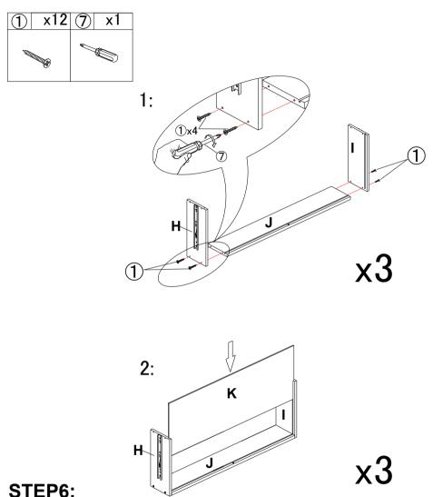
Use screws ① to attach drawer side panel (H)&(I) to drawer back panel (J), and then tighten it with screwdriver ? . Carefully align and slide panel (K) into the groove along rear edge of pre-assembled step 6.1:
