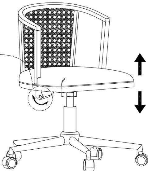
adjust forward and backward tilt angle of chair by rotating rotary knob under chair
