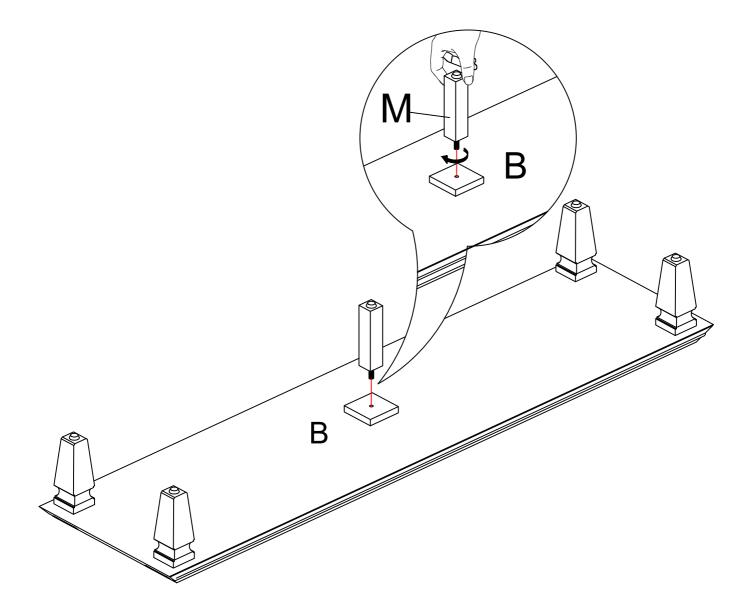
1.Use bolt #15 to attach Weight blocks (P) to bottom panel
