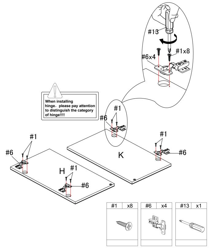
1.Use screw#1 to attach the hinges #7 to door panel (I)&(J), tighten screws with screwdriver #13.
