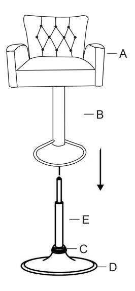
**STEP 3:**Carefully align bottom hole of mechanism with top pin of gas lift then push all the way down to secure.
