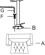
**STEP 2:**Place the chair back A on a clean padded surface, Use bolt F, allen key G to attach mechanism B to bottom of the seat A.
