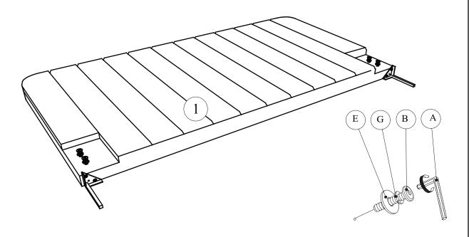
A. Use Allen Key (A) to drive and loossely screw in Bolt (B) fitted with Spring Washer (G) and Flat Washer (E) onto the Headboard Cushion (1).
