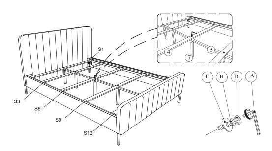
A. With asistance use Bolt (D) fitted with Spring Washer (H) and Flat Washer (F) to fasten Slat (4) #S1 to Center Support Bar (5) and Center Support Leg (7).
