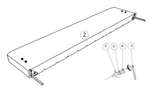
A. Use Allen Key (A) to drive and loossely screw in Bolt (B) fitted with Spring Washer (G) and Flat Washer (E) onto the Footboard Cushion (2).
