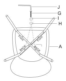
STEP 3: Use bolt G, spring washer I, flat washer H to connect rear holes of legs with bottom of the seat.
