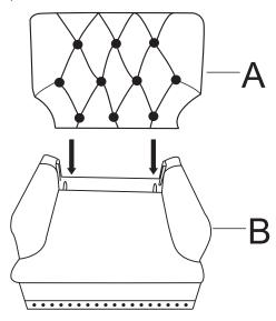
**STEP 2:**Carefully align male and female bracket then push the back all the way down to secure.
