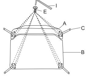
**STEP 3:** Use bolt E, allen key I to attach legs C to bottom of the seat, fasten all bolts to secure.
