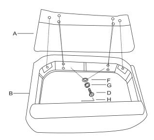
**STEP 2:** Align hole position on seat cushion B and back A, use bolt D, flat washer F, spring washer G, allen wrench H to connect seat and back, make sure bottom edge of back align with rear bottom edge of seat then fasten all bolts to secure.
