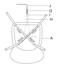
STEP 3: Use bolt G, spring washer I,flat washer H to connect rear holes of legs with bottom of the seat. Make sure all holes on legs align with holes on bottom of seat then fasten all bolts to secure.
