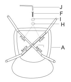
STEP 2: Use bolt F, spring washer I, flat washer H, allen wrench J to attach the Front part of the legs assembly to bottom of the seat.
