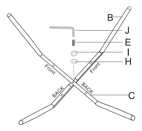
Be sure to check all packing material carefully for small parts, which may have come loose inside the carton during shipment. STEP 1: Use bolt E, spring washer I, flat washer H, allen wrench J to connect metal leg part B and C together, don't fasten the bolt at this stage.
