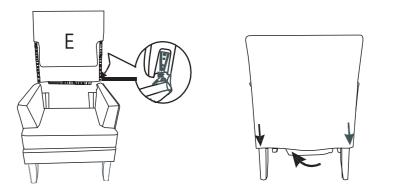
**STEP 4:** Pls insert backrest correctly, then push it down for match up and make sure enough tight. Carefully match the Velcro on back cover then press to secure.
