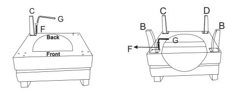
**STEP 2:** Use bolt F, allen key G to attach legs B,C,D to bottom of the seat/back A.
