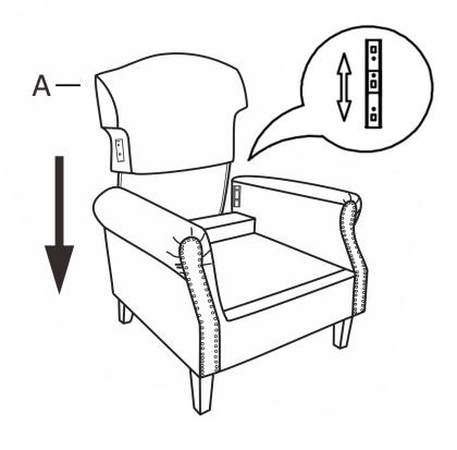
STEP 2: Carefully align male and female metal bracket then push all the way down to secure.
