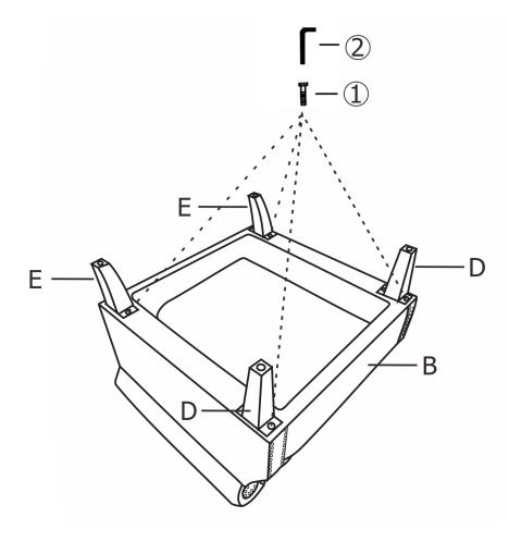
STEP1: Use bolt①, allen key② to attach legs D&E to bottom of the seat, make sure all holes align then fasten all bolts to secure.
