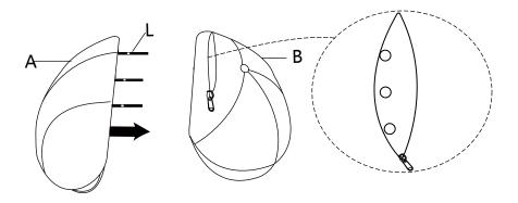
**STEP 3:** Carefully align then insert bolts through holes on edge of chair seat (B)
