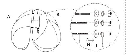
Attach flat washer (J), sping washer (I), hex nut (H) to bolts (L) then fasten to secure.
