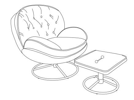
**STEP 8:** Insert the metal base(E) to the small metal base(D)
