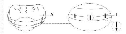
**STEP 1:** place chair back (A) on a clean padded surface, fasten bolt (L) to insert on bottom edge of the chair back (A)
