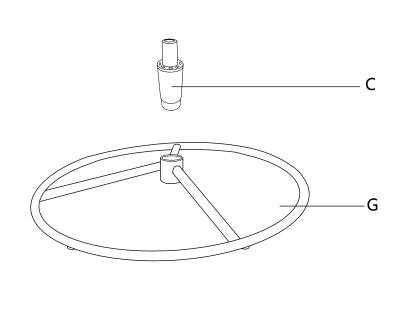
**STEP 5:** Insert lift (C) to the metal base(G)
