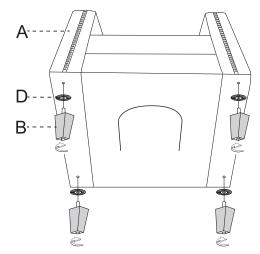
STEP 2 :Attach feet B, rubber washer D to bottom of the base A. Fasten to secure each feet. If any foot doesn't sits parallel with edge of the base please turn harder to make adjustment of the position.
