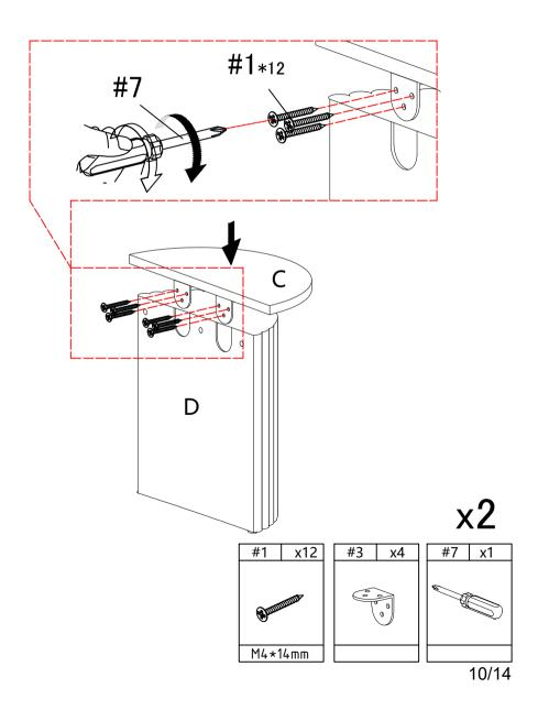
Align the holes in part (C) with the holes in part (D), and tighten screw #1 with screwdriver #7.
