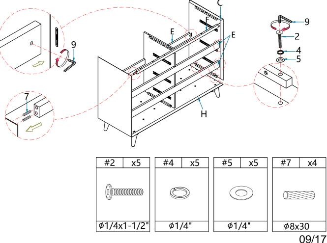
Align the top (A) to left side panel (B), right side panel (C), divider panel (D) then secure by using Wood dowels (7), Bolts (2) and Washers(4,5).
