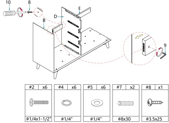
Align left side panel (B) Crossbar front side panel (E) insert the hexagon into the hold and tighten it.
