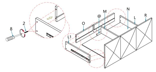
**STEP-10** Insert the Drawer bottom panel (N) to Drawer side panel (L,L1), Drawer back panel (O), Drawer crossbar bottom (@), Drawer crossbar between (M), Drawer panel (P), then secure by using Bolts (2).
