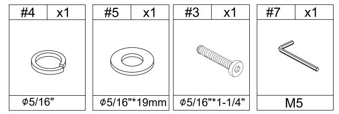
Insert washers #5 and #4 into screw #3 in sequence, install part D on the pre-assembled unit in step 1, make sure the corresponding holes are aligned and secure with screw #3, then tighten screw #3 with an Allen key #7.
