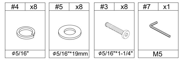
1.Insert gasket #4 and #5 in sequence into bolt #3, install leg (E) on of leg (F), ensure the corresponding holes are aligned and fix with screw #3, then tighten the screw with an Allen key #7.
