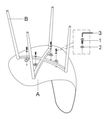
**STEP 1:** Place the chair seat A upside down on clean padded surface, use bolt 1,flat washer 2,allen key 3 to connect leg base B with seat A,make sure all holes aligned and fasten all bolts to secure.
