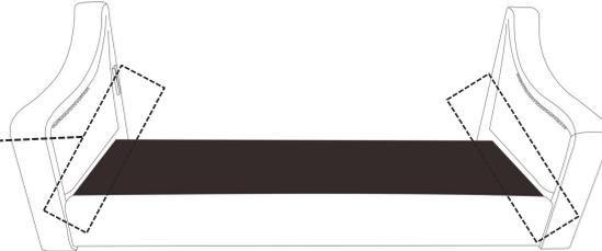
3. Attach the back to the seat and arm as shown, make sure that all the male and female brackets align firmly as shown. (Two person needed here.)
