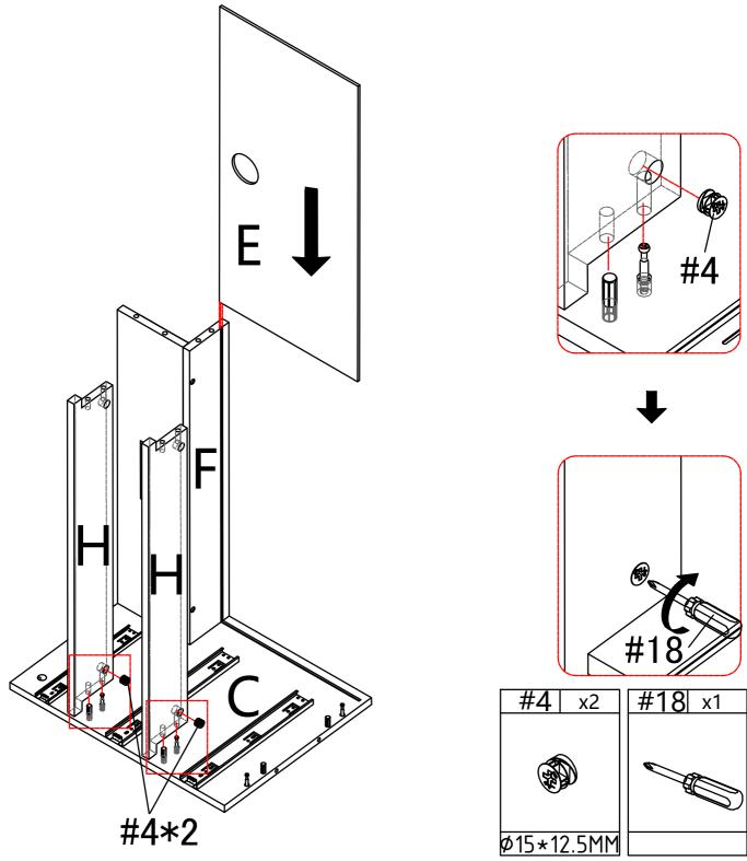
Insert the panels (B) into the side panels (C&E),make sure all holes aligned and insert cam bolt #4 into the corresponding hole of panel (B), tighten cam bolt #4 with screwdriver #18.
