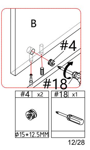
1. insert wood dowel #2 by hand into the corresponding hole in the panel (B&E&H&G)
