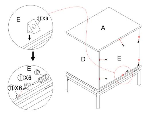
STEP8:Insert hardware ① into part E as shown, screw in screw ① using screwdriver ① and tighten fully.
