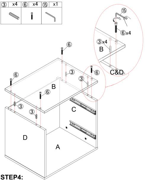
Connect the part B the pre-assembled unit in step 3. Insert the wooden dowel ③ into the part D,C as the picture show. Then align the holes in part B,Insert screw ⑥ and push it down so that it connects to parts C, D. Next,and tighten the screw ⑥ with an Allen key (5). 10/22
