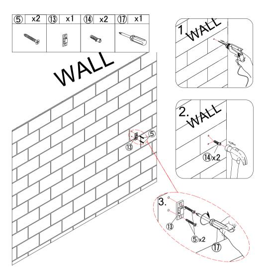
**STEP14:**Mark the position on the wall, that corresponds to the location of part (13) on the side panel A; Drill and insert the expandable screw (14) by hammer.
