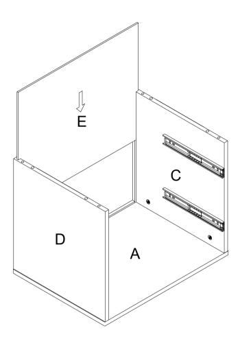
STEP3:slide in the part E into the groove in part C, D . make sure they are also in groove in part A.
