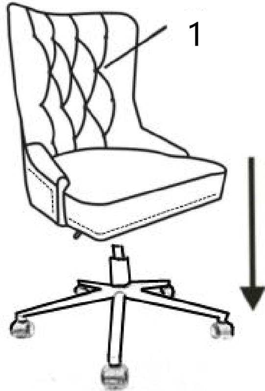
STEP 4: Attach the whole seat to base assembly, make sure top of gas lift align with center hole of mechanism 1 under seat.
