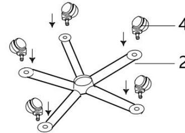
STEP 1: Insert casters 4 to bottom of the spider base 2.
