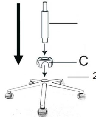
STEP 2: Insert the gas lift 3 and cover C to the center hole of the spider base 2.
