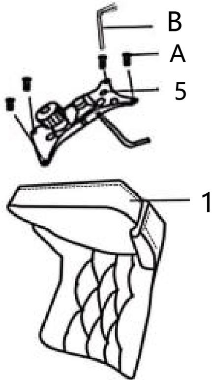
STEP 3: Use bolt A and allen key B to attach mechanism 5 to bottom of the seat 1, make sure the holes align and the arrow in front direction, then fasten bolts to secure.
