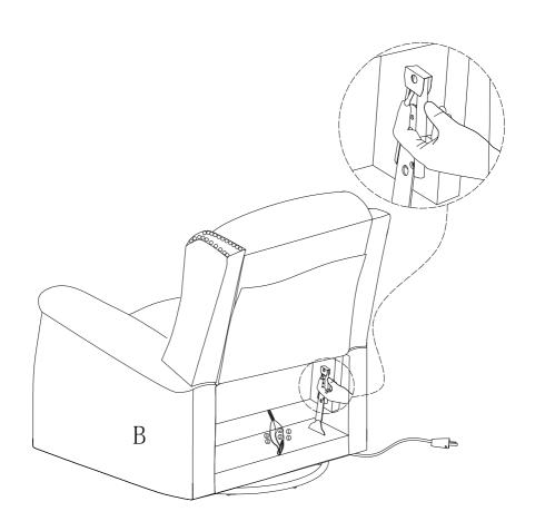
If you need to remove the backrest, please follow the illustration to open the hardware slot switch on one side of the backrest by hand, while pulling it up with force. Do the same on the other side.
