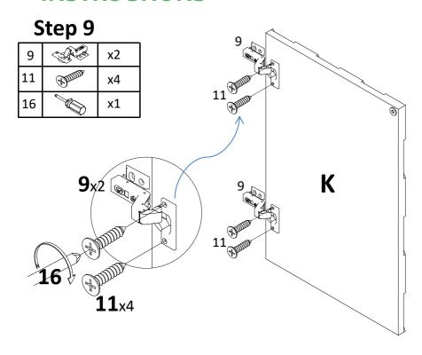
Attach hinge(9) to right door(K) with screw (11). Tight screw with screwdriver(16).
