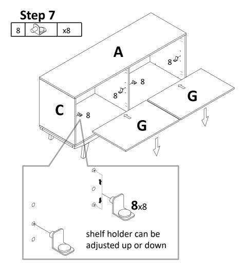
Insert shelf holder (8) to preassemble unit at step 6, and attach adjustable shelf (G) to it.
