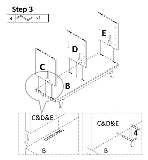
Attach left side panel(C), middle vertical panel(D) and right side panel(E) to bottom panel(B), and tight it with Allen wrench(4).
