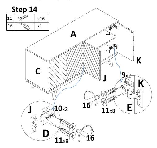
Attach middle right door(J) and right door(K) to preassemble unit at step 13 with screw(11), tight screw with screwdriver(16).
