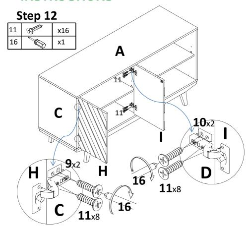
Attach left door(H) and middle left door(I) to preassemble unit at step 7 with screw(11), tight screw with screwdriver(16).
