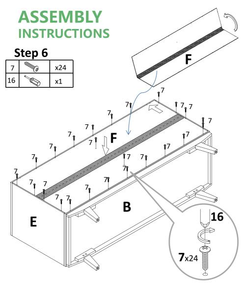
Attach back panel (F) to the unit preassembly unit at step 5 with screw (7), tight screw with screwdriver (16).
