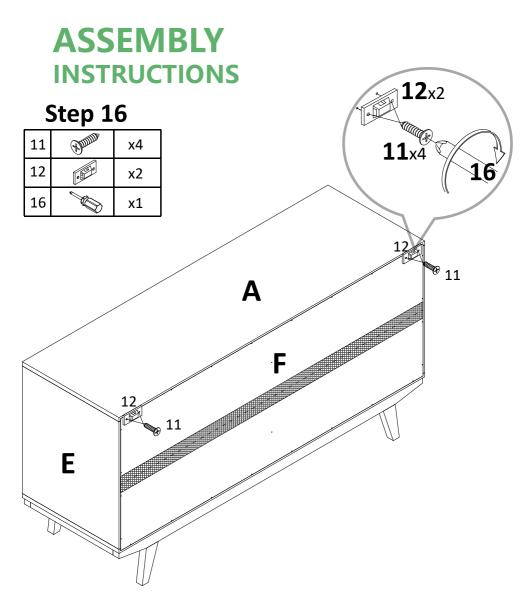
Attach bracket(12) to preassemble unit at step 15 with screw(11), tight screw with screwdriver(16).
