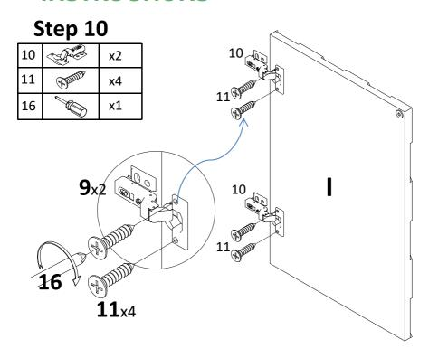
Attach hinge(10) to middle left door(I) with screw (11). Tight screw with screwdriver(16).
