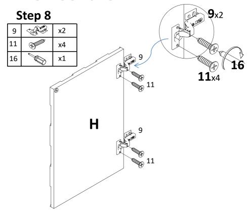
Attach hinge(9) to left door(H) with screw (11). Tight screw with screwdriver(16).
