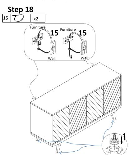
Attach the unit to the wall with plastic belt(15)
