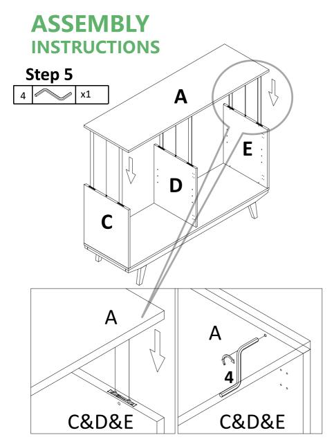
Attach preassemble unit at step 4 to top panel(A), and tight it with Allen wrench(4).
