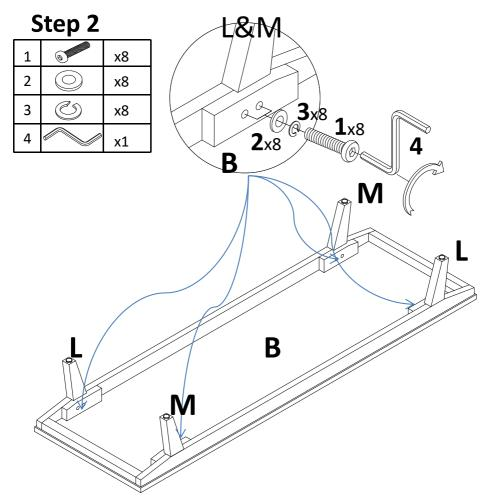
Attach leg(L/M) to bottom panel(B) with bolt(1) ,flat washer(2) and spring washer(3), tight it with Allen wrench(4).
