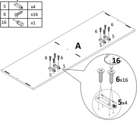
Attach head rebounder(5) to top panel(A) with screw(6) , tight it with screwdriver(16).
