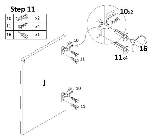
Attach hinge(10) to middle right door(J) with screw (11). Tight screw with screwdriver(16).
