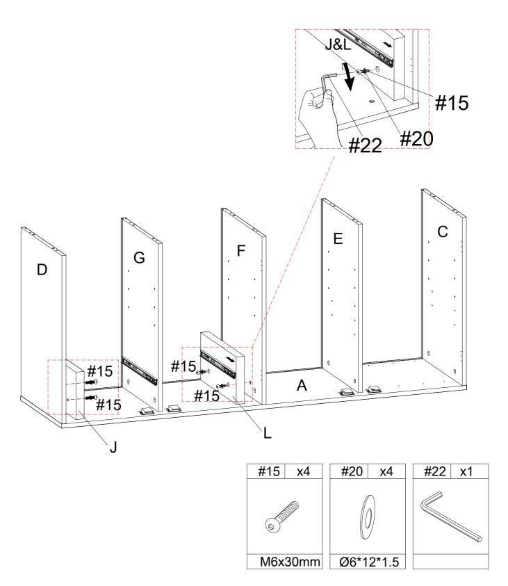
Insert gasket #20 into screw #14. Align the K hole position with the A plate and use the wrench #22 to fix the screw #14 on the A plate respectively
