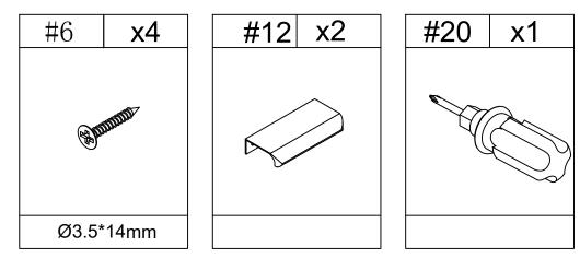
1.Use bolt #6 to attach handle #12 to door panel (J), tighten bolts #6 with screwdriver #20.
