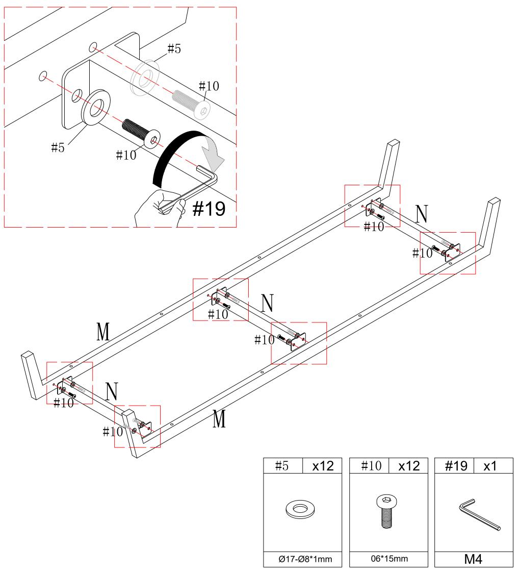
1.connect the leg frame to the cabinet.Attach the leg frame to the pre-assembled unit in step 4 with a screw #11 and tighten #11 with a allen key #19.
