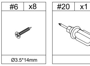
1.Use bolt #6 to attach handle #12 to door panel (I), tighten bolts #6 with screwdriver #20.
