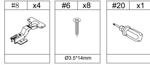
1.Use screw #6 to attach left door (I) and right door (J) to pre-assemble unit at step 7, tighten screw #6 with screwdriver #20.
