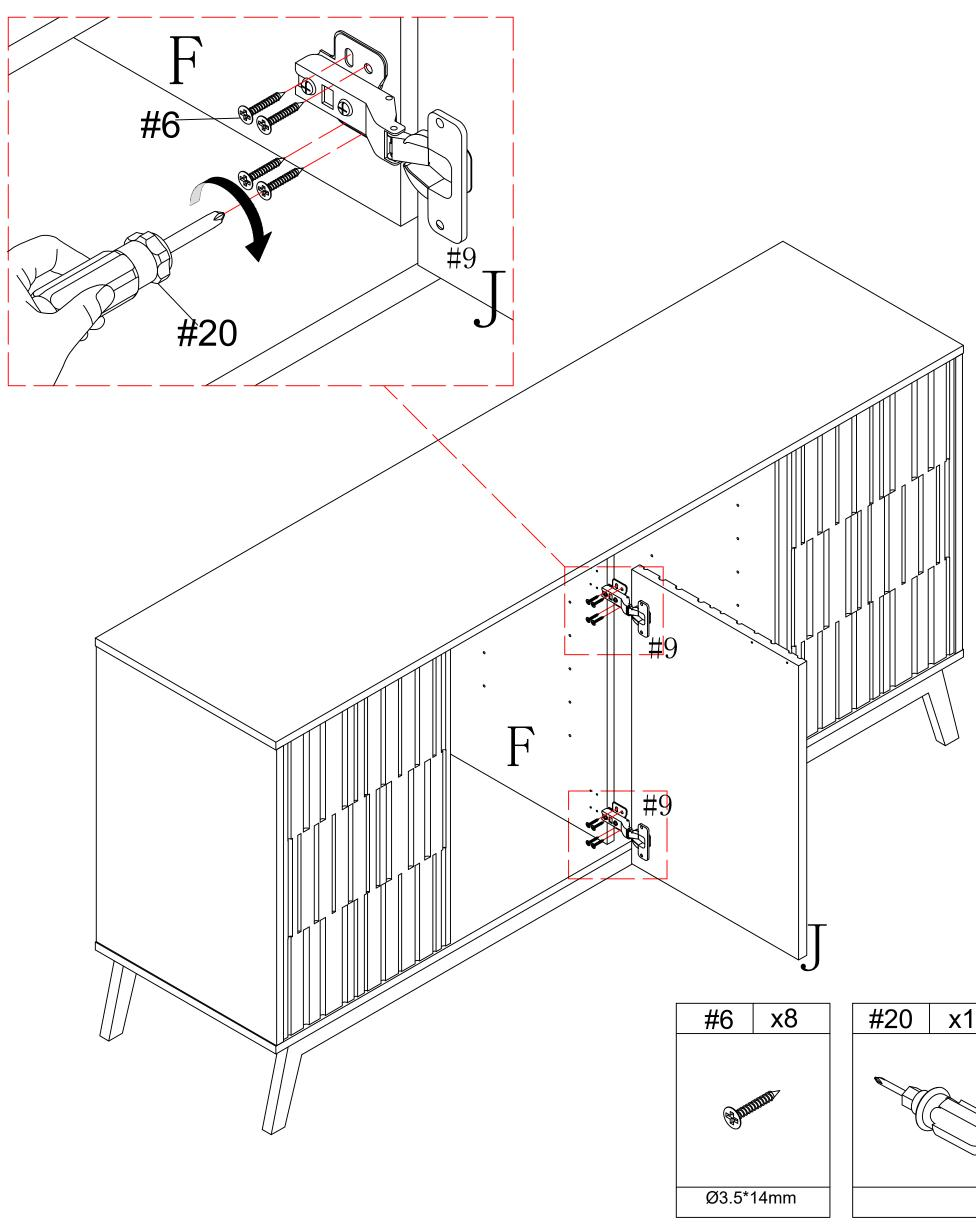
1.Use screw #6 to attach middle door (I) to pre-assemble unit at step 11 ,tighten screw #6 with screwdriver #20 .
