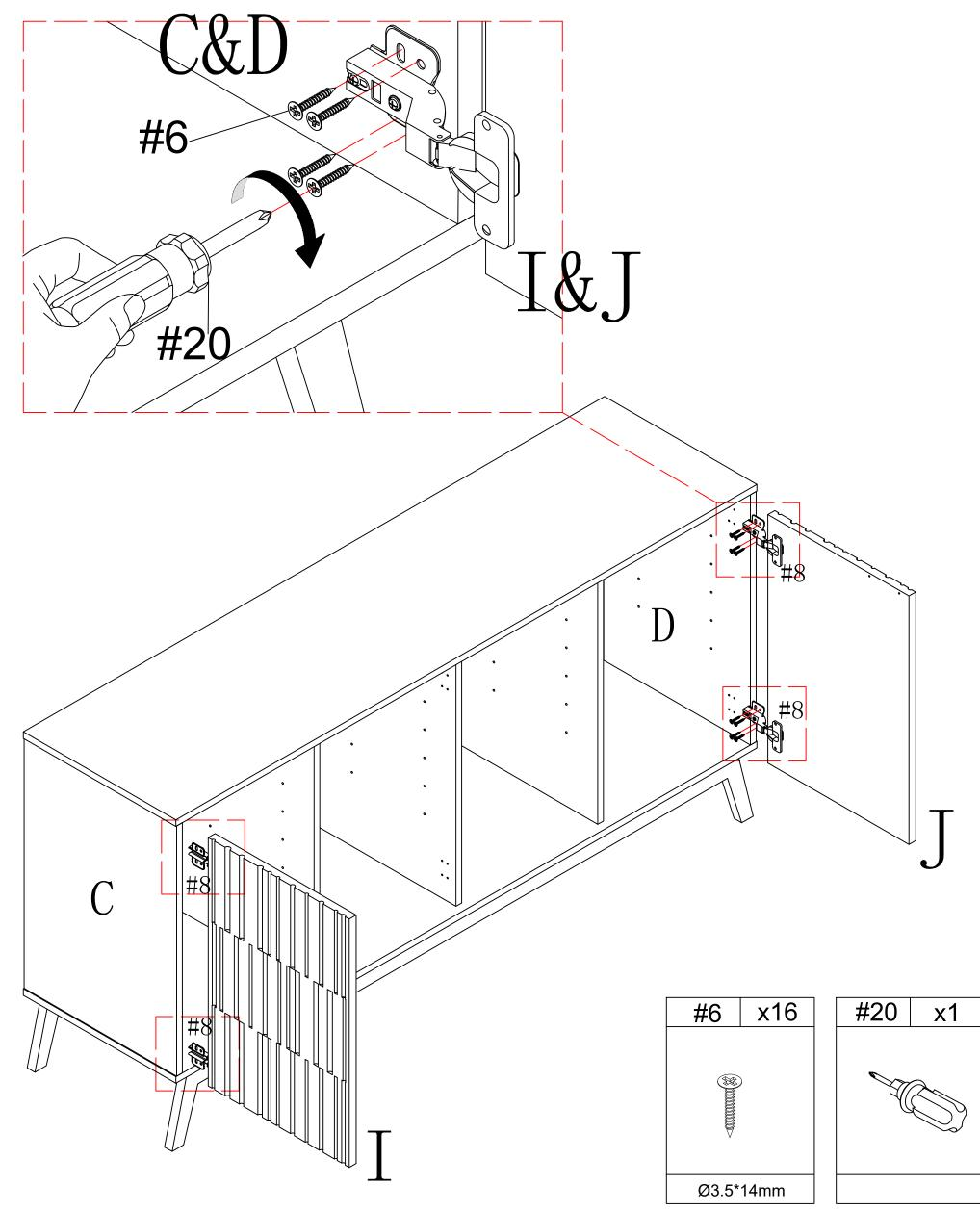
1.Use screw #6 to attach the hinges #9 to door panel (I&J), tighten screws #6 with screwdriver #20.
