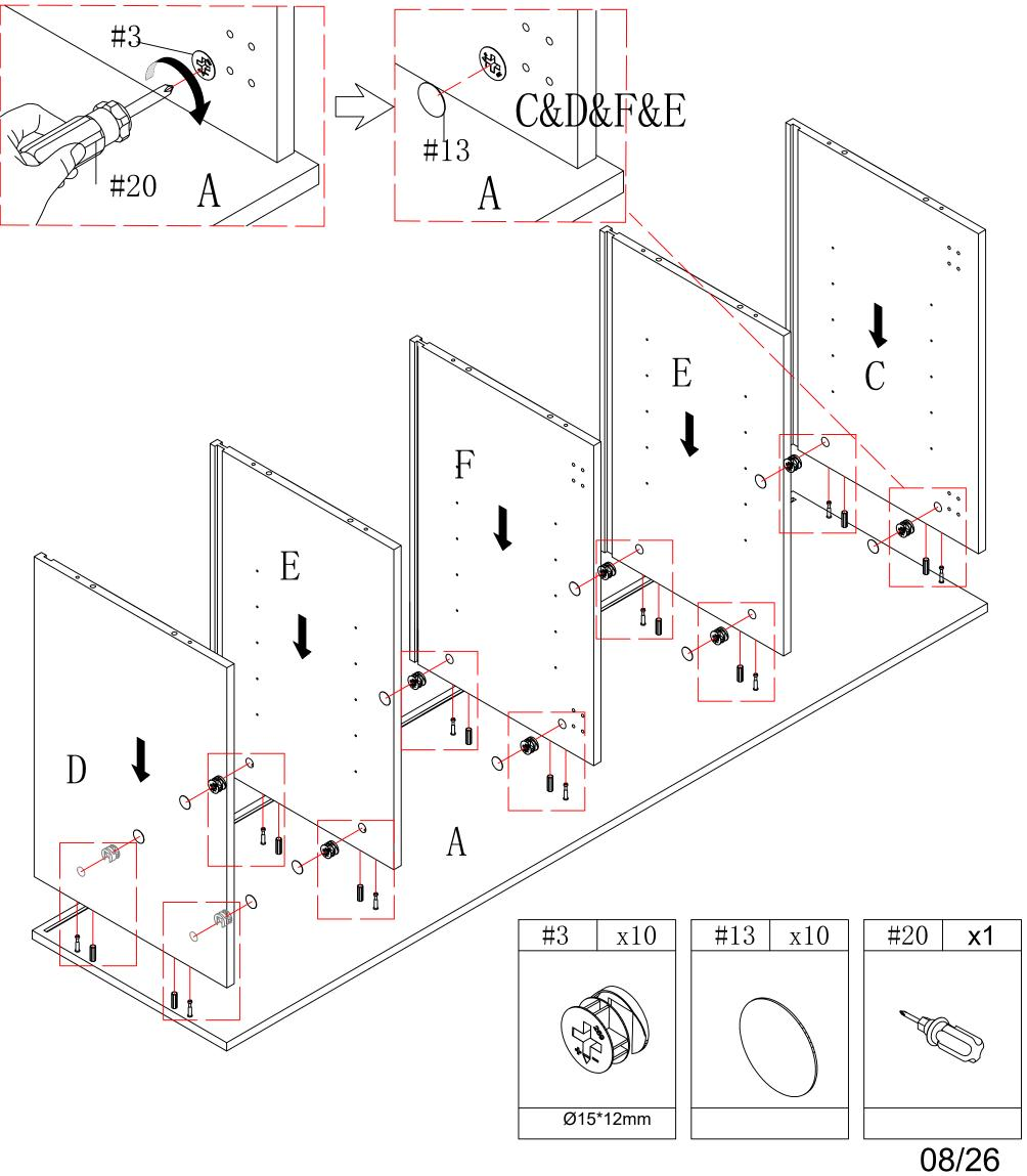
1.slide in the part L,K into the groove in part D,E and E,F and F,E,and C,E . make sure they are also in groove in part A.Insert the wooden dowel #2 into the part C&D&E&F as the picture show.
