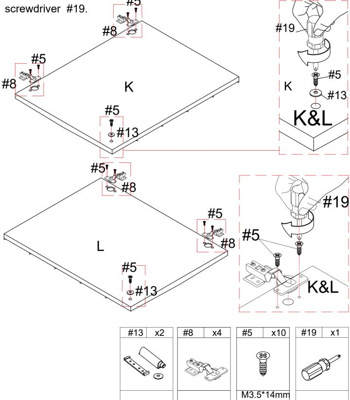
1.Use screw #5 to attach left door (K) and right door (L) to pre-assemble unit at step 10 ,tighten screw #5 with screwdriver #19
