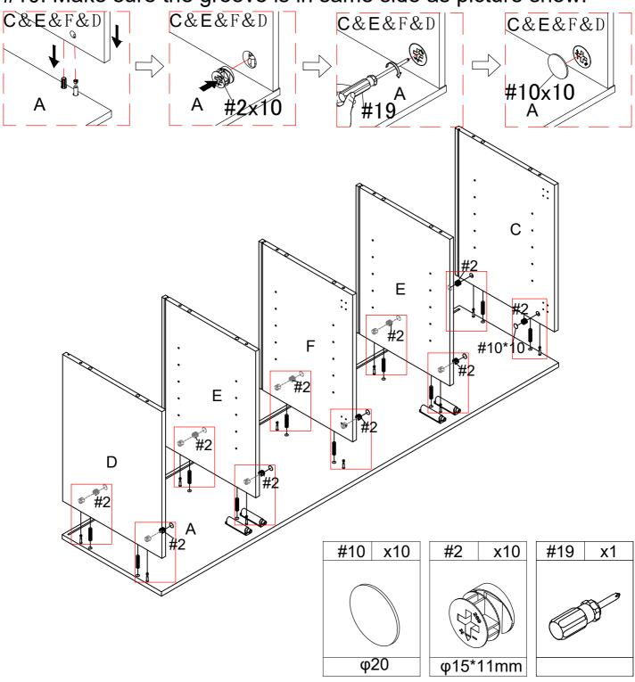
1.slide in the part J,I into the groove in part D,E and E,F and F,E,and C,E . make sure they are also in groove in part A.
