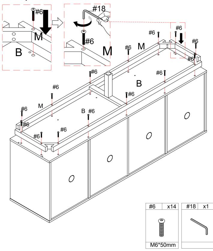
1.install leg N on of part M , ensure the corresponding holes are aligned and fix with screw #6, then tighten the screw with an Allen key #18.
