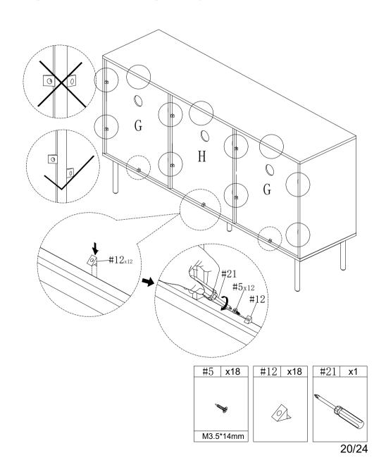
1.Use screw #5 to attach part #16 to pre-assemble unit at step 14 ,tighten screws with screwdriver #21.
