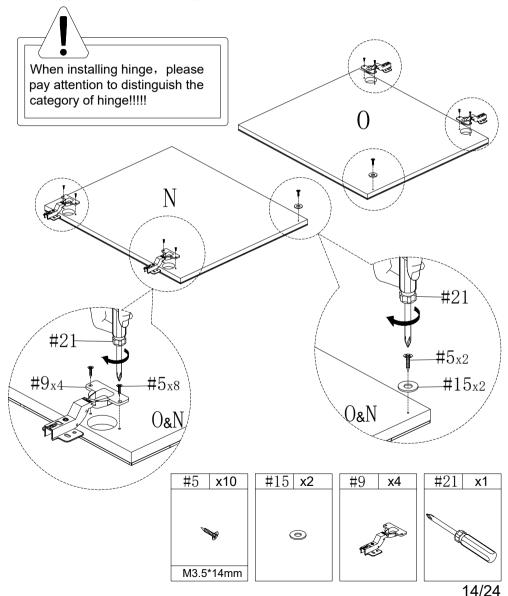
1.Use screw #5 to attach left door (N) and right door (O) to pre-assemble unit at step 8 ,tighten screw #5 with screwdriver #21 .
