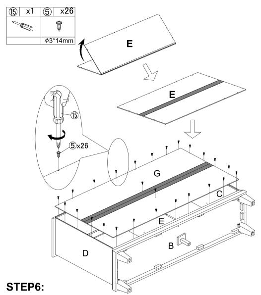
Insert back panel (G) into the groove of preassemble step 5, make sure all holes aligned, and then use screw (5) to attach back panel (G) to preassemble step 5, tighten screw (5) with screwdriver(15).
