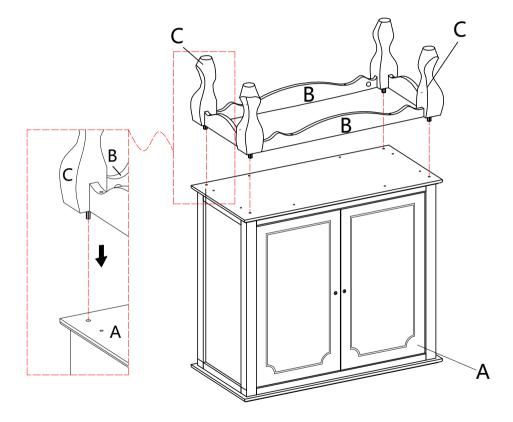
In preassemble step 3, make sure all holes aligned and then use bolt #4 to attach them, tighten bolt #4 with screwdriver #10.
