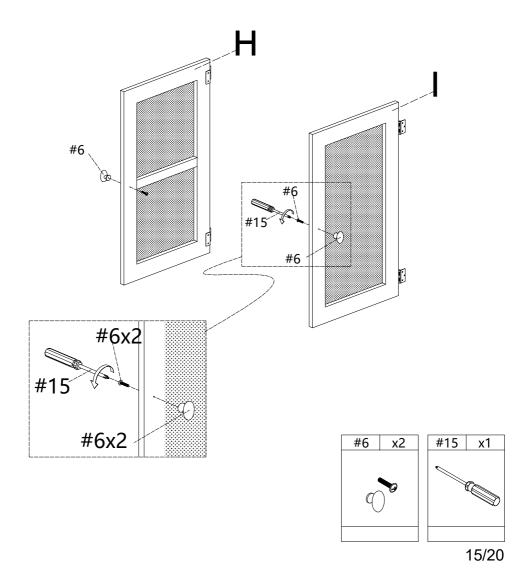
Use screw#5 to attach preassemble door(H)&(I) to the corresponding hole of side panel(C)&(D) as picture show,tighten it with screwdriver#15.
