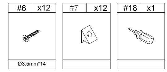
1.Use screw #6 to attach the hinges #8 to door panel (G), tighten screws #6 with screwdriver #18.
