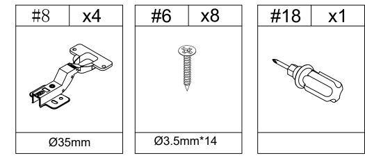
1.Use screw #6 to attach left door (G) and right door (G) to pre-assemble unit at step 8, tighten screw #6 with screwdriver #18.
