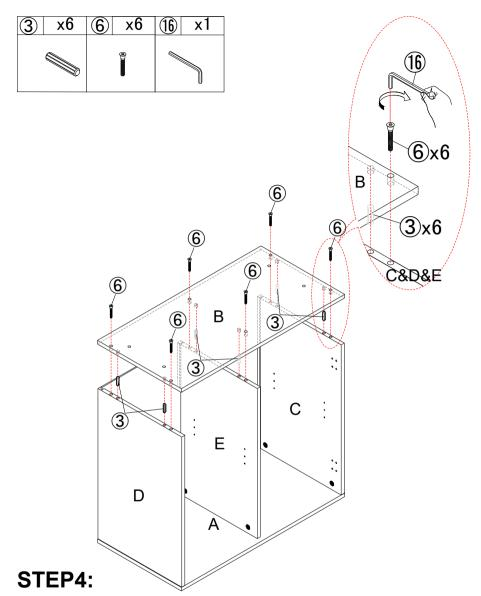
Insert wooden dowel 3 into the corresponding hole of panel (C)&(D)&(E),and then insert bottom panel (B) into the preassemble step3, make sure all holes aligned and use bolt 6 to attach them, tighten bolt 6 with allen key 16.
