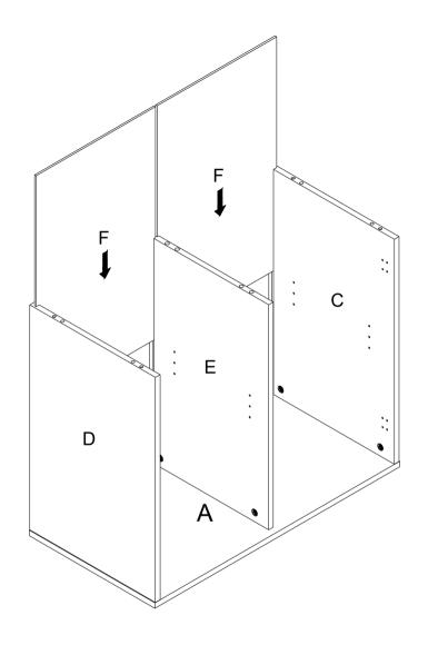
**STEP3:**Carefully align and slide panel (F) into the groove along rear edge of pre-assembled step 2.
