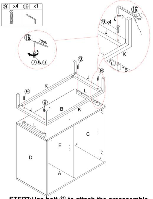
STEP7:Use bolt (9) to attach the preassemble leg(J)&(K) to the corresponding hole of part (L),tighten bolt (9) with allen key (6).
