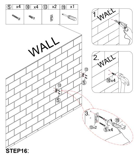
Mark the position on the wall, that corresponds to the location of part (1) on the side panel D,C; Drill and insert the expandable screw (1) by hammer.
