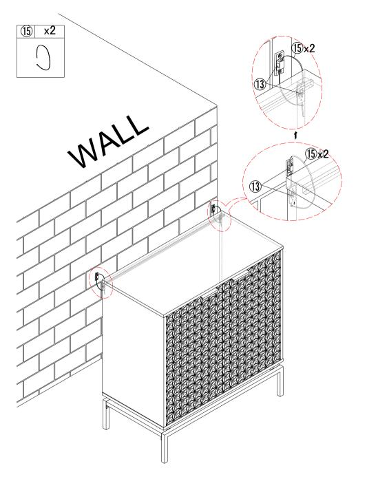
**STEP17:** Let the plastic belt (15) pass through the both part (13) and pull tightly.
