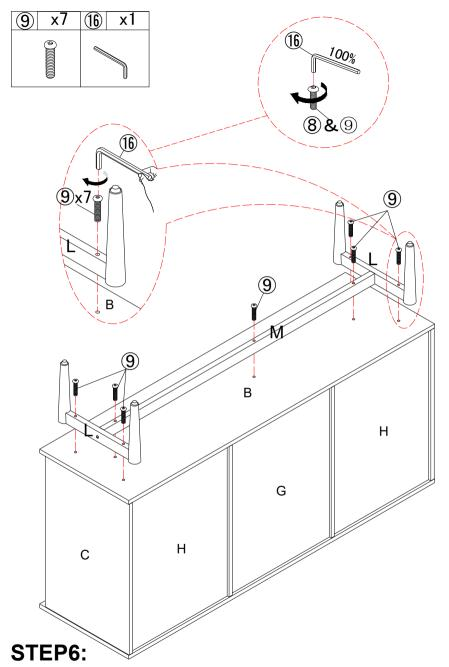
connect the leg frame to the cabinet. Attach the leg frame to the pre-assembled unit in step 4 with a screw (9) and tighten (9) with a allen key (16).
