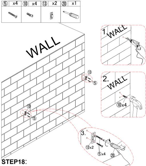
Mark the position on the wall, that corresponds to the location of part (13) on the side panel D&C; Drill and insert the expandable screw (10) by hammer.
