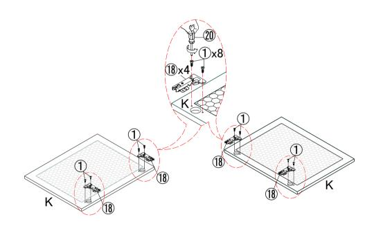
STEP11:Use screw ① to attach the hinges ® to door panel (K), tighten screws ① with screwdriver ②.
