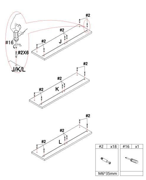
Insert drawer panel(J)&(K)&(L) into the corresponding hole of preassemble step 12.2, make sure all holes aligned and insert cam bolt #4 into drawe panel(E)&(F),tighten cam bolt #4 with screwdriver #16.
