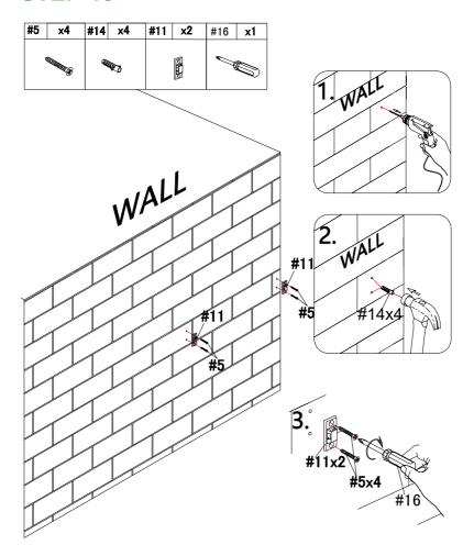
**STEP20:**Mark the position on the wall, that corresponds to the location of part #11 on the side panels C,D; Drill and insert the expandable screw #14 by hammer.
