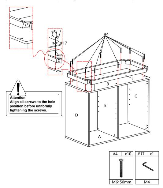
Use bolt #4 to attach leg (K) to the corresponding hole of part (B) as picture show, tighten bolt #4 with allen key #17.
