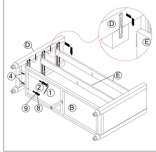
Step 4.A.Attach the center panel (F) to the base panel (B) by placing the plastic pieces in the slots and sliding the center panel (F) forward.
