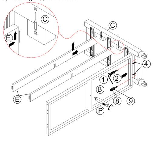
Step 3A.Attach the right side panel (D) to the beams (E) by placing the plastic pieces in the slots and sliding the right side panel (D) backwards.
