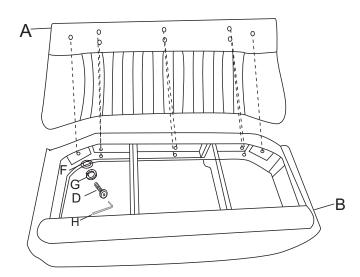
**STEP 2** Align hole position on seat cushion B and back A, use bolt D, flat wahser F, spring wahser G allen wrench H to connect seat and back, Don't fasten any bolt until all botls connected properly and position aligned correctly.
