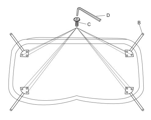
**STEP 2**: Use bolt C, allen key D to connect the metal leg B to bottom of the seat cushion A, make sure all holes algin, fasten all bolts to secure.
