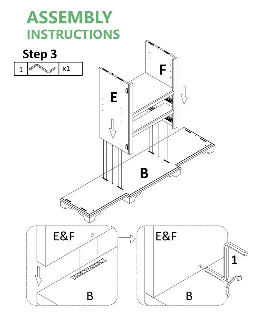
Attach preassemble unit at step 2 to bottom panel(B), and tight it with Allen wrench(1).
