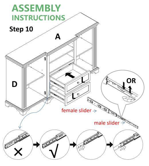
Make sure to move the ball bearing to front end, carefully align male and female slides before insert drawer box.
