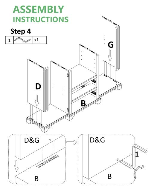
Attach left side panel(D) and right side panel(G) to preassemble unit at step 3, and tight it with Allen wrench(1).
