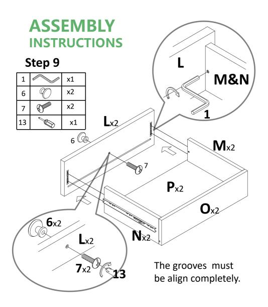
Attach drawer front (L) to preassemble unit at step8, tight it with allen wrench(1).
