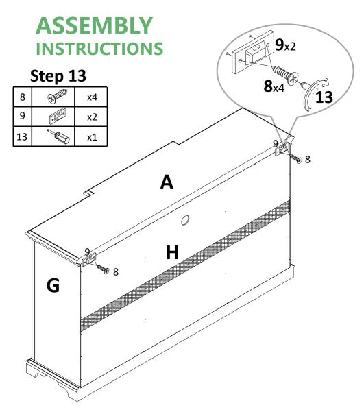
Attach bracket(9) to preassemble unit at step 12 with screw(8), and tight screw with screwdriver(13).
