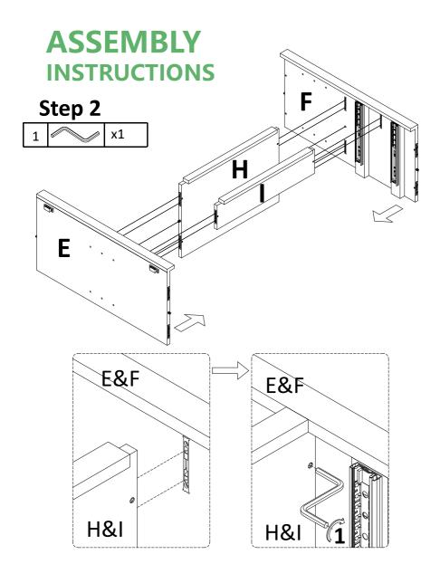
Attach fixed shelf panel (H) and front rail(I) to middle vertical panel left(E) and middle vertical panel(F) as image. And tight them with allen wrench(1).
