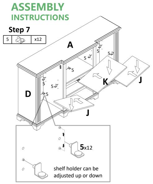
Insert shelf holder(5) to preassemble unit at step 6, and attach adjustable shelf (K/J) to it.
