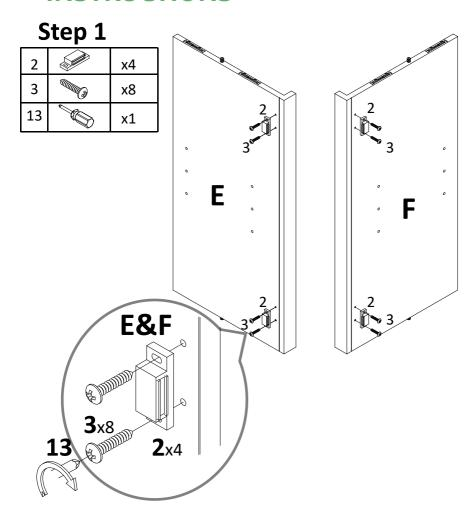
Attach magnet (2) to middle vertical panel left(E) and middle vertical panel right(F) with screw(3). Tight screw with screwdriver(13).
