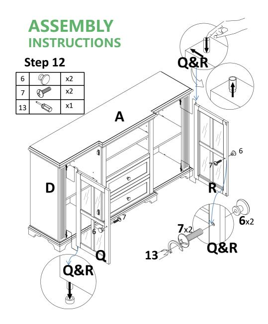
Attach left door(Q) and right door(R) to preassemble unit at step 11, attach konb(6) to left door(Q) and right door(R) with bolt(7), tight bolt with screwdriver(13).
