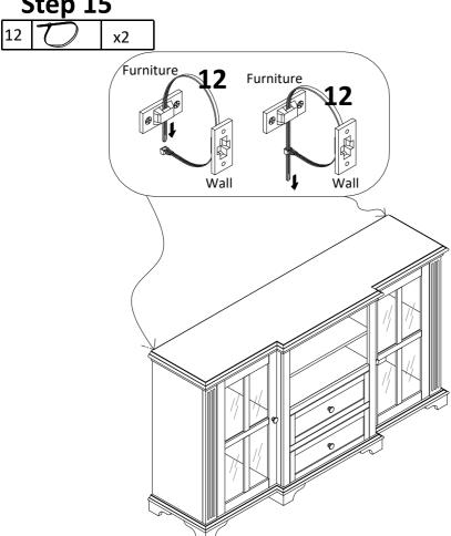
Attach the unit to the wall plastic belt(12)
