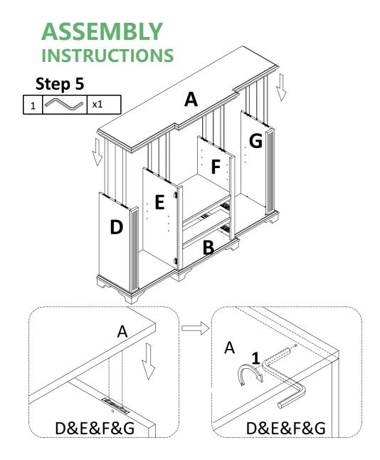
Attach top panel(A) to preassemble unit at step 4 and tight it with Allen wrench(1).
