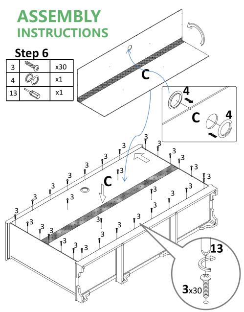
Attach plastic circle(4) to back panel(C). Attach back panel(C) to the preassemble unit at step 5 with screw (3), tight screw with screwdriver(13).
