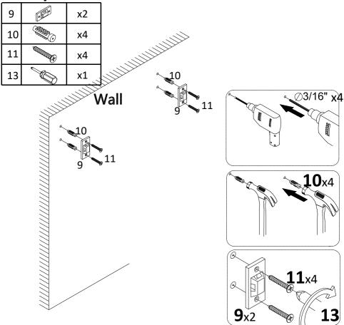
Drill hole on the wall, and insert expansion nut(10), then attach bracket(9) to it with screw(11), tight screw with screwdriver(13).
