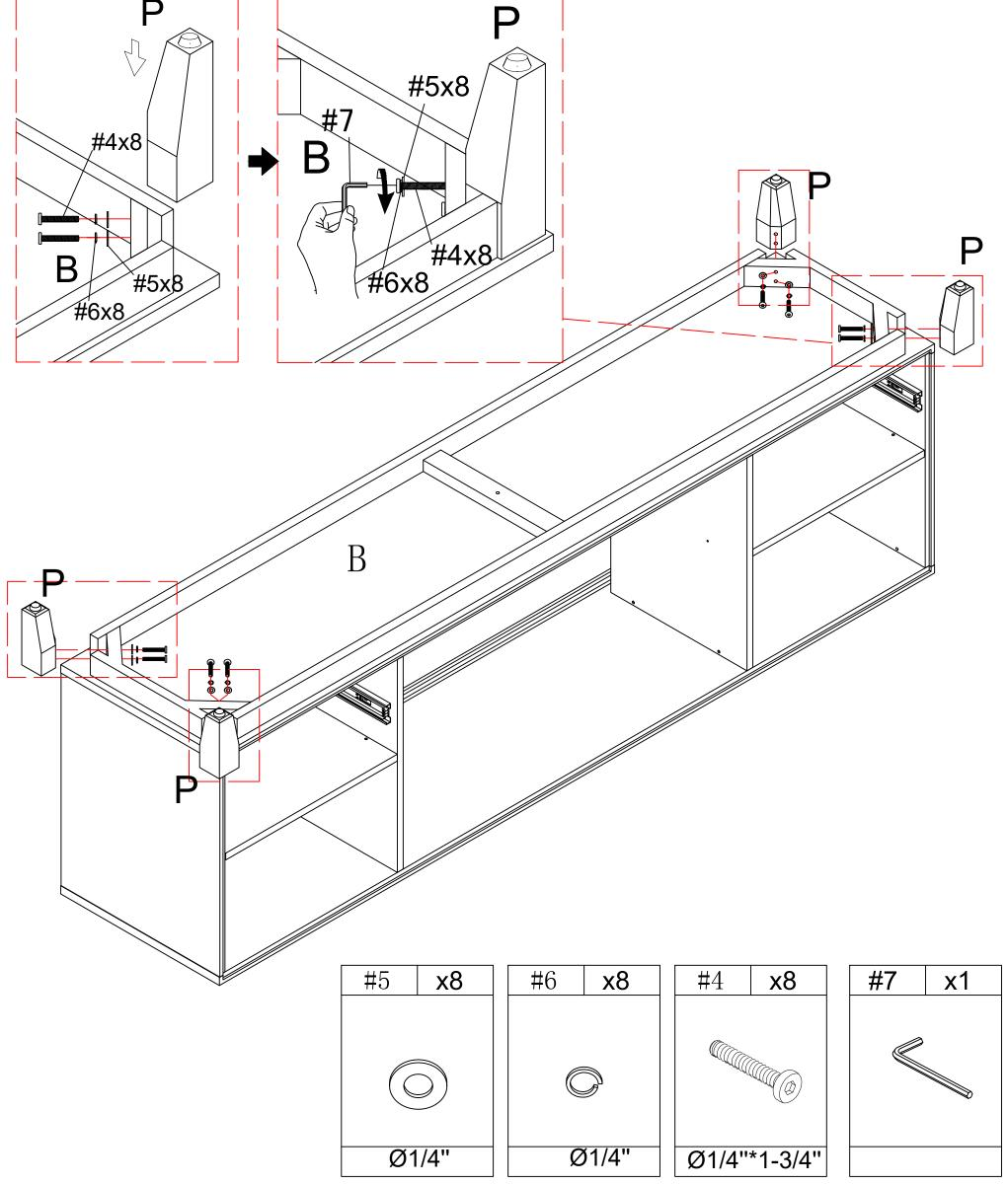
1.Install the mid-foot to base plate B.
