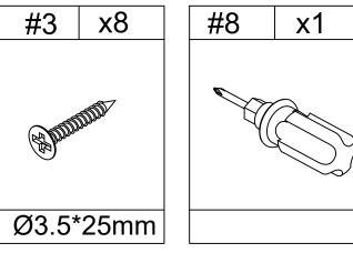
1.Connect the (M) and (K&J) using screw #3 , and tighten it with screwdriver #8.
