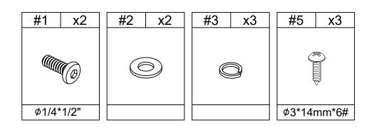
1.connect part(M/N) to part (B) with bolt #1, flat washer #2 and spring washer #3, tight them with allen wrench #11.
