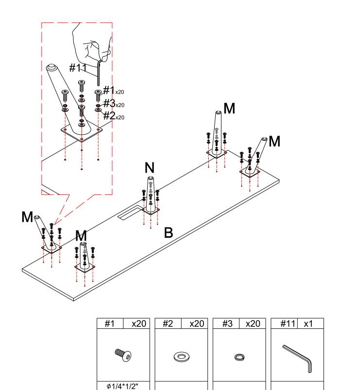
1.insert part(C/F) to part (B), make sure all holes aligned and tight it with allen wrench #11.
