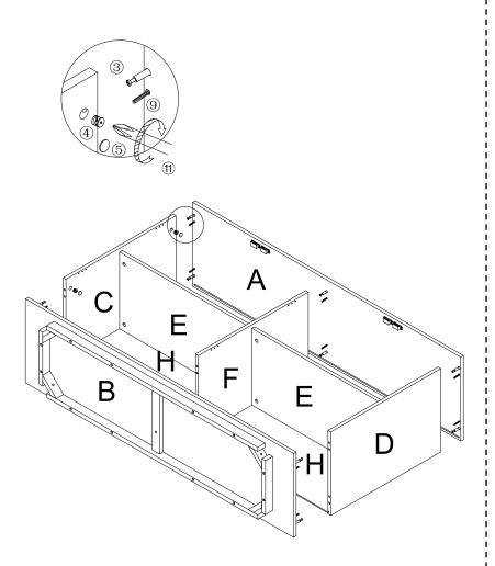
STEP 6: Insert cam bolt #3 and dowel #9 on part A/B through end hole of part C/D/F, use philips head screwdriver #11 to fasten cam bolt #4 for secure part A/B with part C/D/F.Apply sticker #5 to cover the cam nut.
