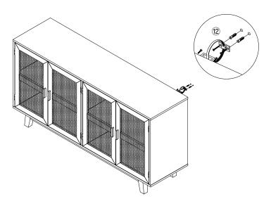
STEP 11: Attach tipping kits to the wall and backside of the unit.
