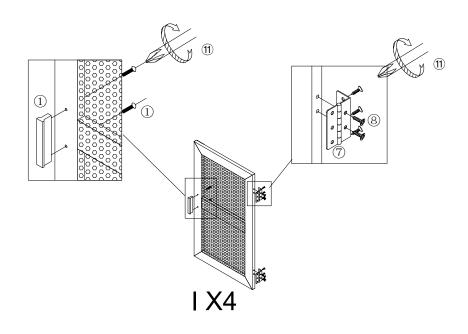
STEP 9: Use philips head screwdriver #11 and screw #8 to attach hinge #7 to part I, then use philips head screwdriver #11 and screw to attach handle #1 to door I.
