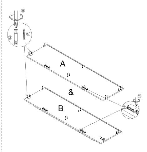
STEP 5: Use philips head screw driver #11 to fasten cam bolt #3 and insert dowel #9 on part A/B, then use screw #2 to attach magnetic catch to pilot hole on part A/B.
