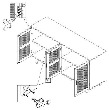
STEP 10: Attach the metal plate# 2 on the panel I with screw#2 by screwdriver#11.
