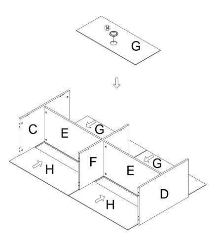
STEP 4: Insert gromet ring #14 into hole of part G, then slide part G/H into groove on part E/F.
