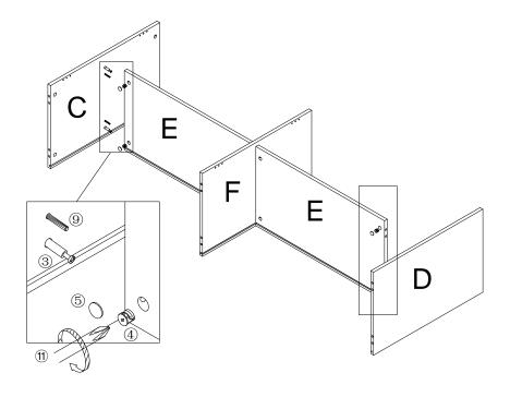
STEP 3: Insert cam bolt #3 and dowel #9 on part C/D through end hole of part E, use philips head screwdriver #11 to fasten cam bolt #4 for secure part C & D.Apply sticker #5 to cover the cam nut.
