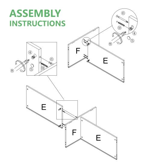
STEP 1: With help of adult partner, hold part F , insert cam bolt #6 through and dowel #9 into dowel hole of part F, then insert cam bolt #6 and dowel #9 through end hole of part E, then insert cam nut #4 and use philips head screwdriver #11 to fasten cam bolt #4 for secure part E & F. Apply sticker #5 to cover the cam nut.
