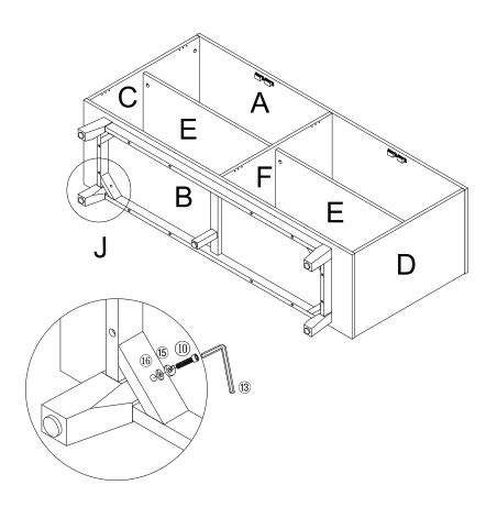
STEP 8: Use allen key #13, bolt #10, spring washer #15, f lat washer #16 to attach leg #J to apron of part #B, fasten all bolts to secure.
