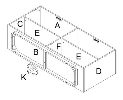
STEP 7: Turn the leg K and fasten it on bottom of part B.
