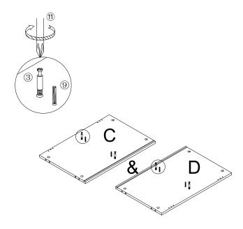
STEP 2: Use philips head screwdriver #11 to fasten cam bolt #3 and insert dowel #9 into part C & D.
