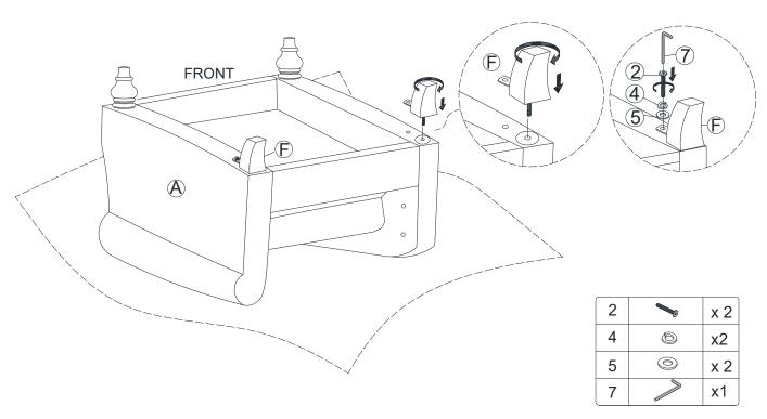
Be sure the wood leg with metal piece-C is aligned tightly, and the hole of the metal piece is matching the hole of the arm bottom.
