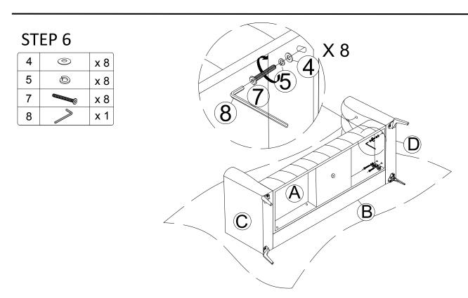
Put on the Washers (5)&(4) to Long Bolt (7), then make sure the Long Bolt (7) go through the hole from the Seat Frame(A), to the holes from Arm(C) &(D), then tighten completely by the Allen wrench (8).
