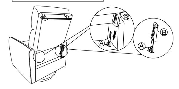
Attach the Back (B) to the seat frame (A) by sliding the receivers into the mechanism posts located on the seat frame (A).
