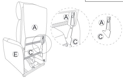
Attach the Back (A) to the seatframe (C) by sliding the receivers into the mechanism posts located on the seatframe (C).
