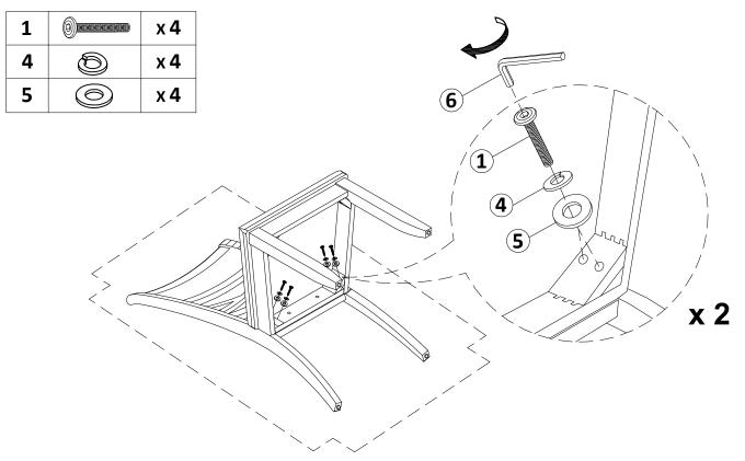
Use Bolt (1), Spring Washer (4) and Flat Washer (5), tighten Bolt (1) by Allen Wrench (6) as shown.
