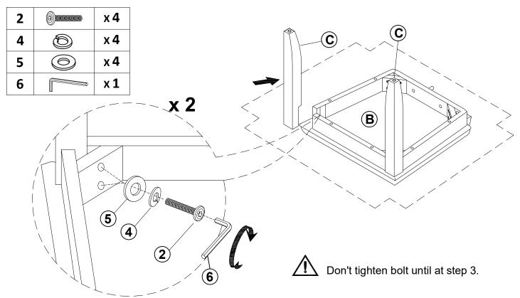
Attach the Front Leg (C) to Seat Frame (B), use the Bolt (2), Spring Washer (4) and Flat Washer (5), tight Bolt (2) with Allen Wrench (6) as shown.
