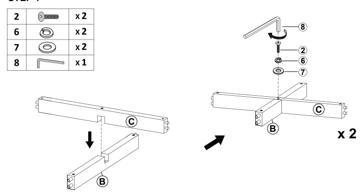
Attach the Connecting Rod (C) to Connecting Rod (B)by align the slot . then use bolt (2) and spring washer (6) and flat washer (7) and Allen Wrench (8) to tighten, As shown.
