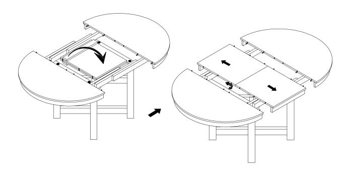
Pull out the active folding small top panel to unfold.
