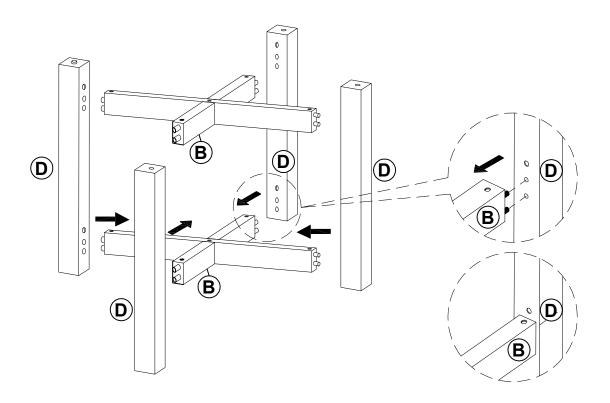
Insert the wooden dowels at both ends of bottom connection (B/C) into the correct holes of the Leg (D).
