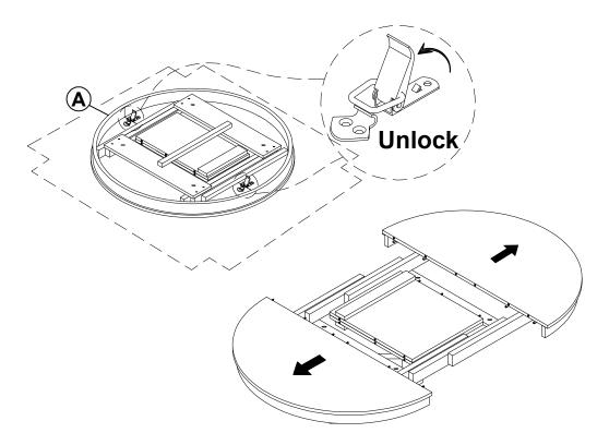
Open the buckle at the bottom of the desktop, pull the side panels outward.
