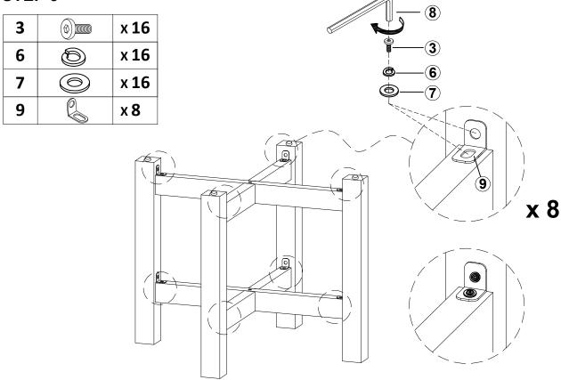
Use Bolt (3), Spring Washer (4) and Flat Washer (5), L Connector (8), tighten Bolt (3) by Allen Wrench (8) as shown.
