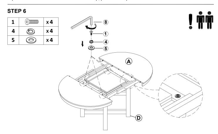
Attach the Table Top (A) on the unit pre-assembled on step 4, and then align the foot frame holes with the holes on the connecting plate below the Table Top (A) and use the hardware (1 and 4 and 5) to fix the panel (A) and the foot frame.
